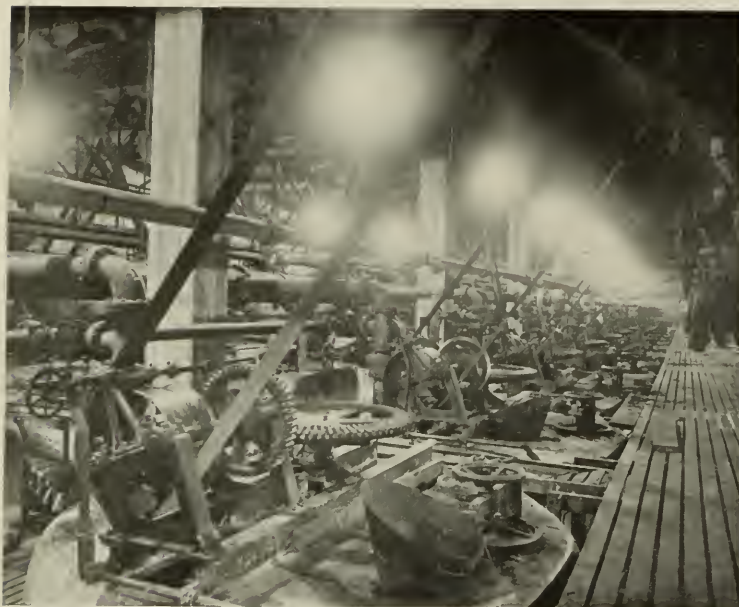
Fig. 2. Night View of Reducers showing Maze of Steam Piping and Belting, and in spite of these, the Excellent Illumination that has been Obtained
