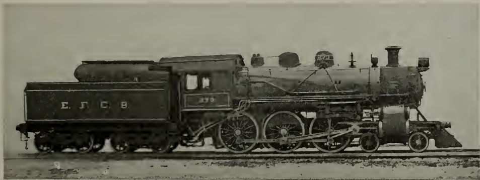
Ten-wheel Locomotive in Service on Central Railway of Brazil Cylinders ..... 21½ inches x 20 inches Driver wheels ..... 68 inches Weight on drivers ..... 124,200 pounds Boiler pressure ..... 175 pounds
