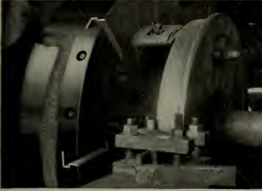
Fig. 11. Cast Iron Head of Car Wheel Lathe Repaired by Electric Arc
