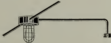
Fig. 4. Plug Attachment for Portable Light for Cleaning and Repairing Reducers. These outlets are located on either side of the Lighting Units shown in Fig. 5
