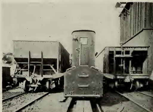
Fig. 13. 25-ton "Pusher" Locomotive with Both Pusher Arms in Operating Position
