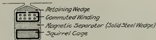
Fig. 11. Inductively Responsive Magnetic Bridge Between the Two Rotor Windings
