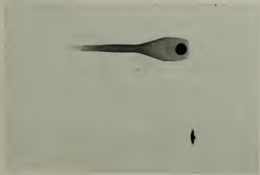
Fig. 14. Lower, Roentgenogram of Target of Tube shown in Fig. 13; Upper, Roentgenogram of Target of Standard Tube
