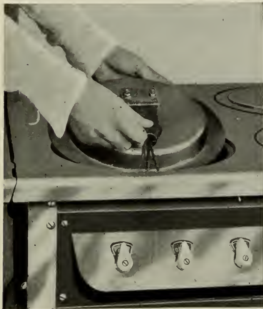
Fig. 6. Method of Attaching Plug to Hot Plate
