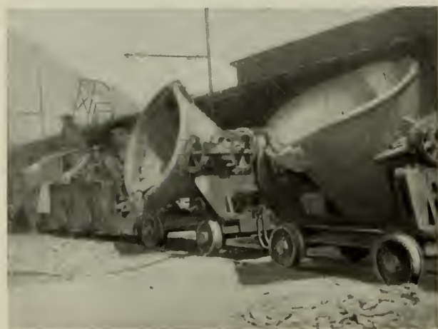
Fig. 6. Electric Locomotive Handling Slag, Casapalca, Peru
