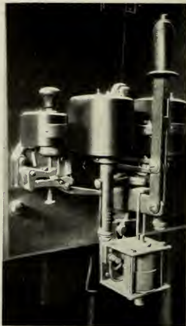
Fig. 9. Toggle Tripping Mechanism of Oil Switch, Operated by Device Shown in Fig. 8
