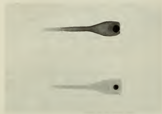
Fig. 9. Lower, Roentgenogram of Hooded Target; Upper, Roentgenogram of Target of Standard Tube
