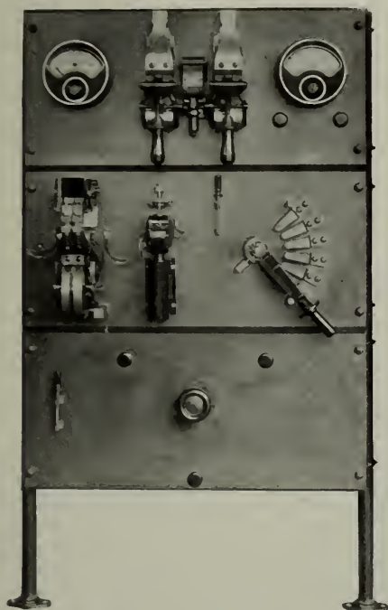
Fig. 20. Arc Welding and Generator Control Panel
