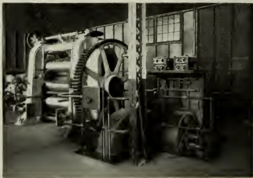
Fig. 31. Motor-driven Rubber Calender Equipped with Automatic Push Button Control
