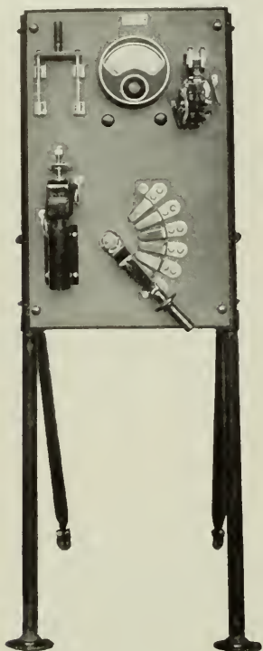
Fig. 22. Auxiliary Arc Welding Panel
