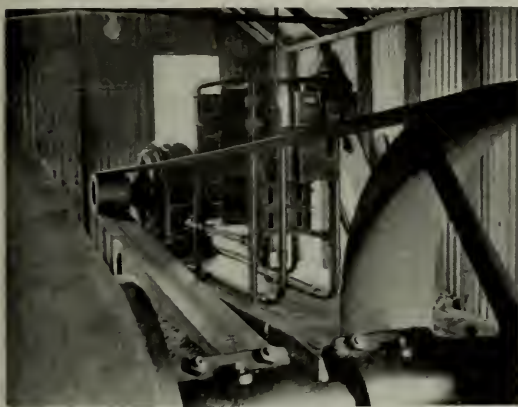
Fig. 7. A Kansas installation of a two-speed variable-speed oil-well motor equipment for pumping, pulling and cleaning work
