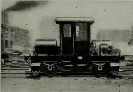
Fig. 15. 12-ton Locomotive Showing Arrangement of Compressors and Air Storage Tanks
