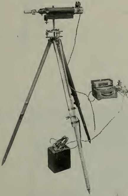
Fig. 1. Portable photometer and accessories
