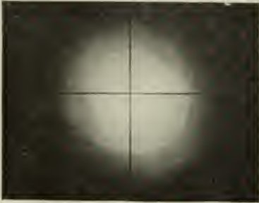
Fig. 5. Screen image of beam projected by parabolic reflector. The bulb is at the focus of the parabola
