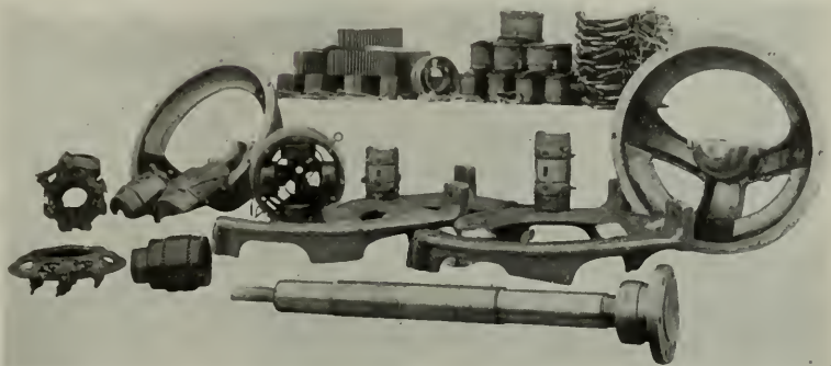
Fig. 4. Parts of a 120 Kw. Alternator and Direct Connected Exciter Constructed for Muleback Transportation, no part of which weighs more than 300 Lb.
