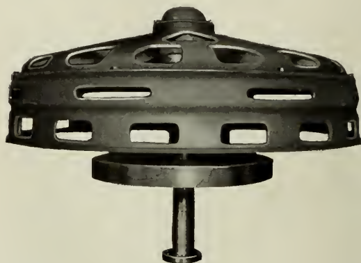
Fig. 8. 150-kv-a., 120-r.p.m. Waterwheel Driven Generator
