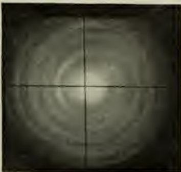
Figs. 7 and 7a. Screen image, bulb in front of focus
