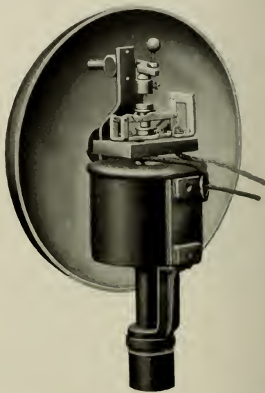
Fig. 10. Counter-Gong Relay for Spark-tube Discharge Alarm
