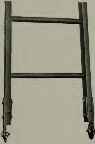
Non-slip device for ladders. Sharp toothed wheel may be adjusted when teeth become worn
