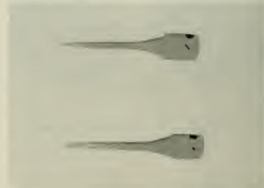
Fig. 11. Lower, Roentgenogram of Hooded Target; Upper, Roentgenogram of Hooded Target with Tungsten Foil
