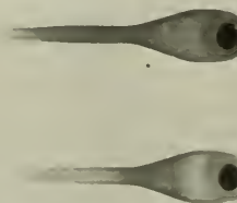
Fig. 5. Roentgenograms showing the effect of voltage. Upper, 10-in. Spark Gap; Lower, 2-in. Spark Gap
