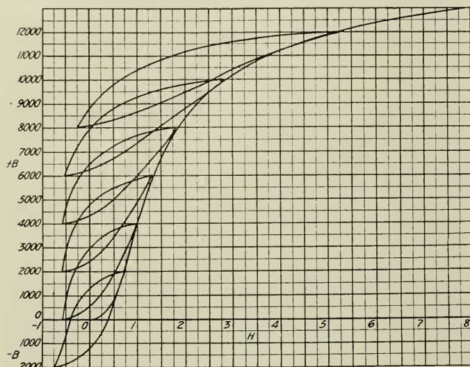
Fig. 7. Group of unsymmetrical hysteresis curves of amplitude B = \pm 2000 , starting at various flux densities along the magnetic saturation curve of silicon steel and then returning to the starting point
