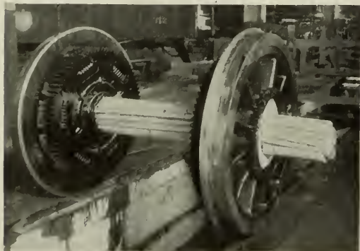
Pair of Driving Wheels, showing Method of Protecting Axle
