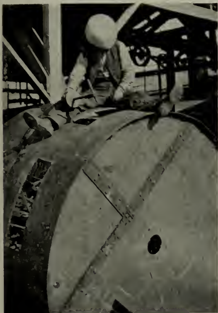
Shell for Steel Furnace showing tuyere openings and bolt holes cut by arc. The position of a new electrode in the holder is clearly shown
