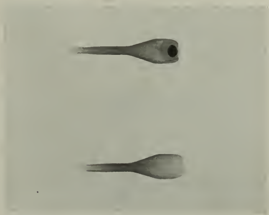
Fig. 3. Roentgenograms of Front and Back of Target. Note that, except for Working Face, Intensity is Practically the same Front and Back
