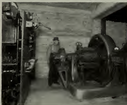
Fig. 21. 300 kw. Motor-generator Set for Electric Metallurgical Processes, which Consists of a 4000 Ampere Direct-current Generator Driven by a 450-h.p. Squirrel-cage Induction Motor
