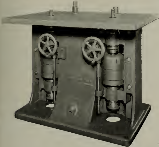
Fig. 13. Double Spindle Shaper with Motor Built-in
