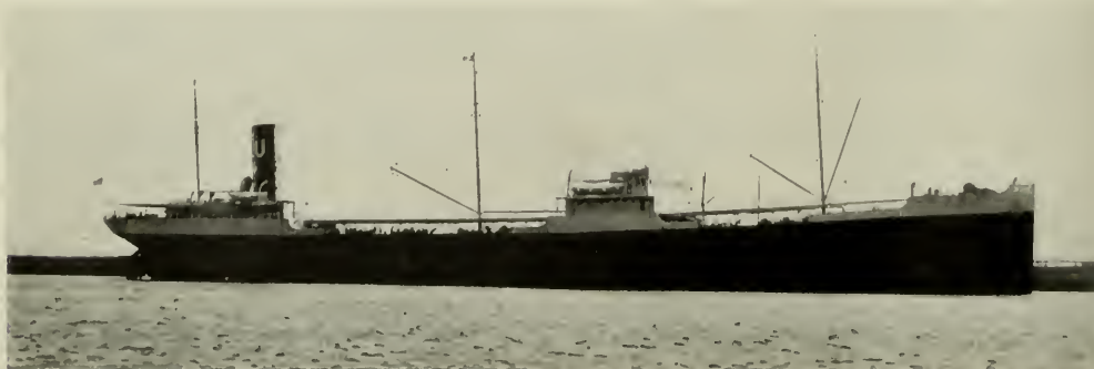
Fig. 5. Steamship "La Brea" Powered with 2600-h.p. Curtis Turbine Driving through Alquist Reduction Gear
