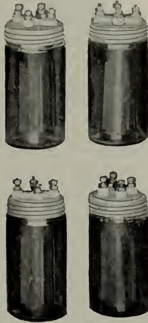
Fig. 4. Aluminum Rectifier Cells for Providing 125-volt Direct Current where no Other Source of Direct Current is Available
