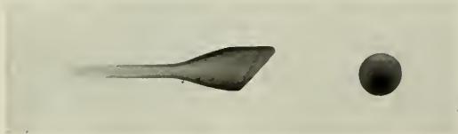
Fig. 17. Right, Roentgenogram of Target of Tube shown in Fig. 16; Left, Broadside View of Target for Comparison
