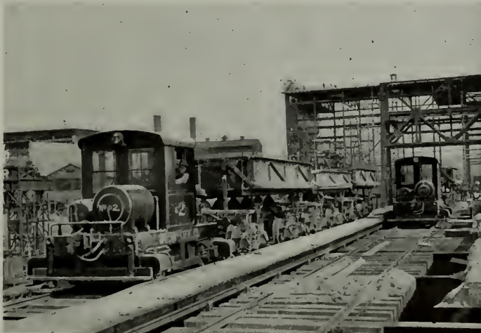
Fig. 16. Two 20-ton Locomotives Hauling Trips, Showing the Over-running Third Rail and Current Collectors
