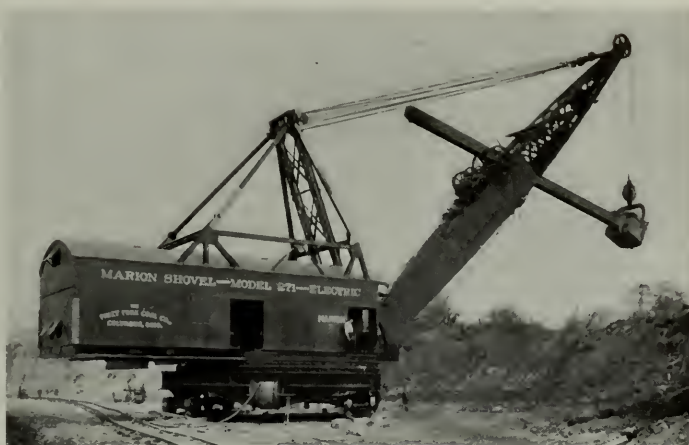
Fig. 19. 250-ton Electric Stripping Shovel in Coal Field at Smithfield, Ohio
